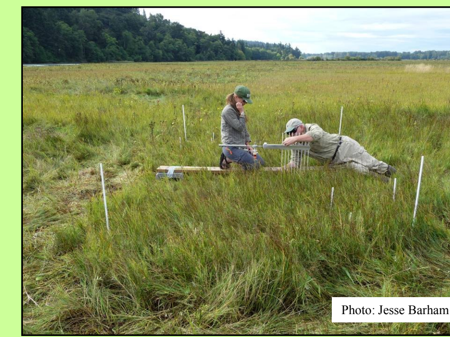
Glenn Guntenspergen and Kelley Turner using Surface Elevation Table to measure elevation changes.
